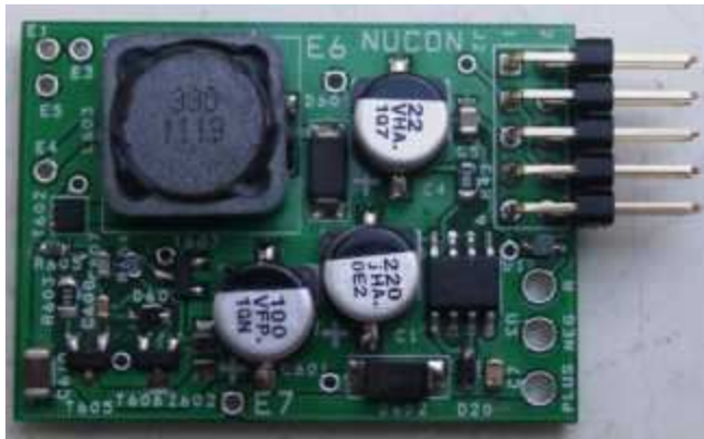
BUCK regulator based on PIC 18F
